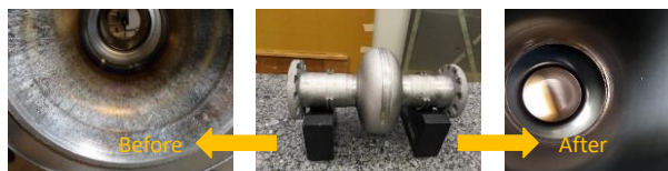
Figure 11. The niobium 1.3 GHz cavity treated by MMP technology.
