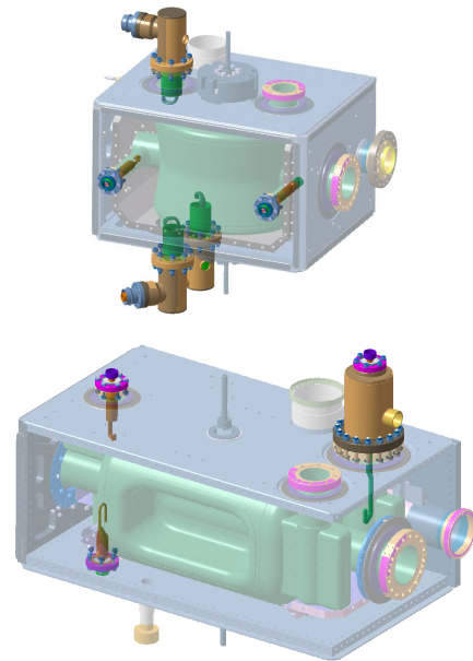
Figure 1: 3D views of the DQW (top) and RFD (bottom) dressed crab cavities with RF couplers and antennas.
