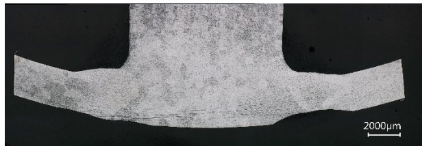
Figure 10: Macrograph of welding test sample used to qualify the Nb-Nb hooks' welds.
